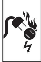
Do not remove the grounding pin from any plug and always make sure all wiring to the machine is grounded before operating. Any electrical outlet and circuit that you plug your machine into must be grounded. Serious injury may occur if this warning is ignored!
